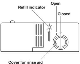
Open by turning and lifting the cover!
